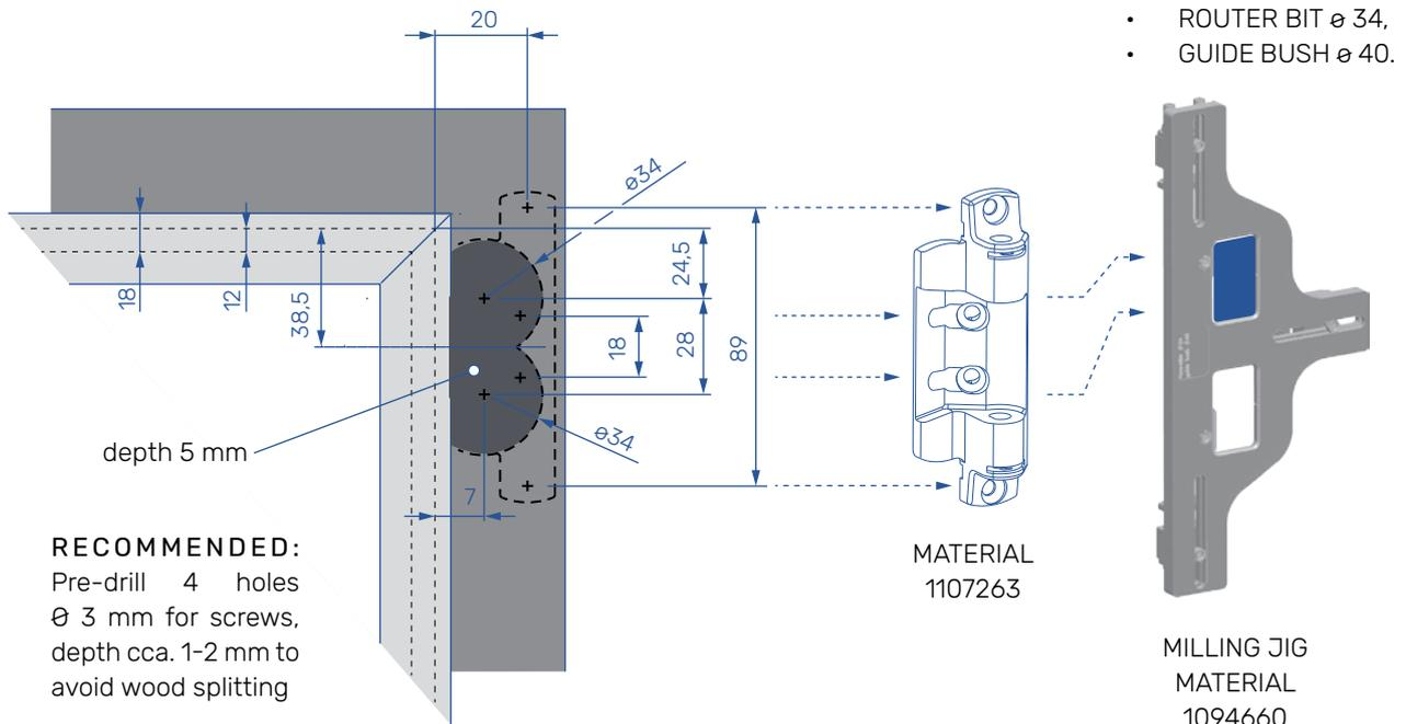
\* READJUST THE MILLING JIG TO 18 mm HARDWARE OVERLAP
