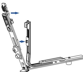
2.) Clamp the hole of a driving rod onto the tilt lock bolt connector
