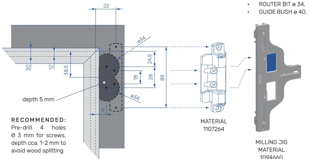
\* READJUST THE MILLING JIG TO 20 mm HARDWARE OVERLAP
