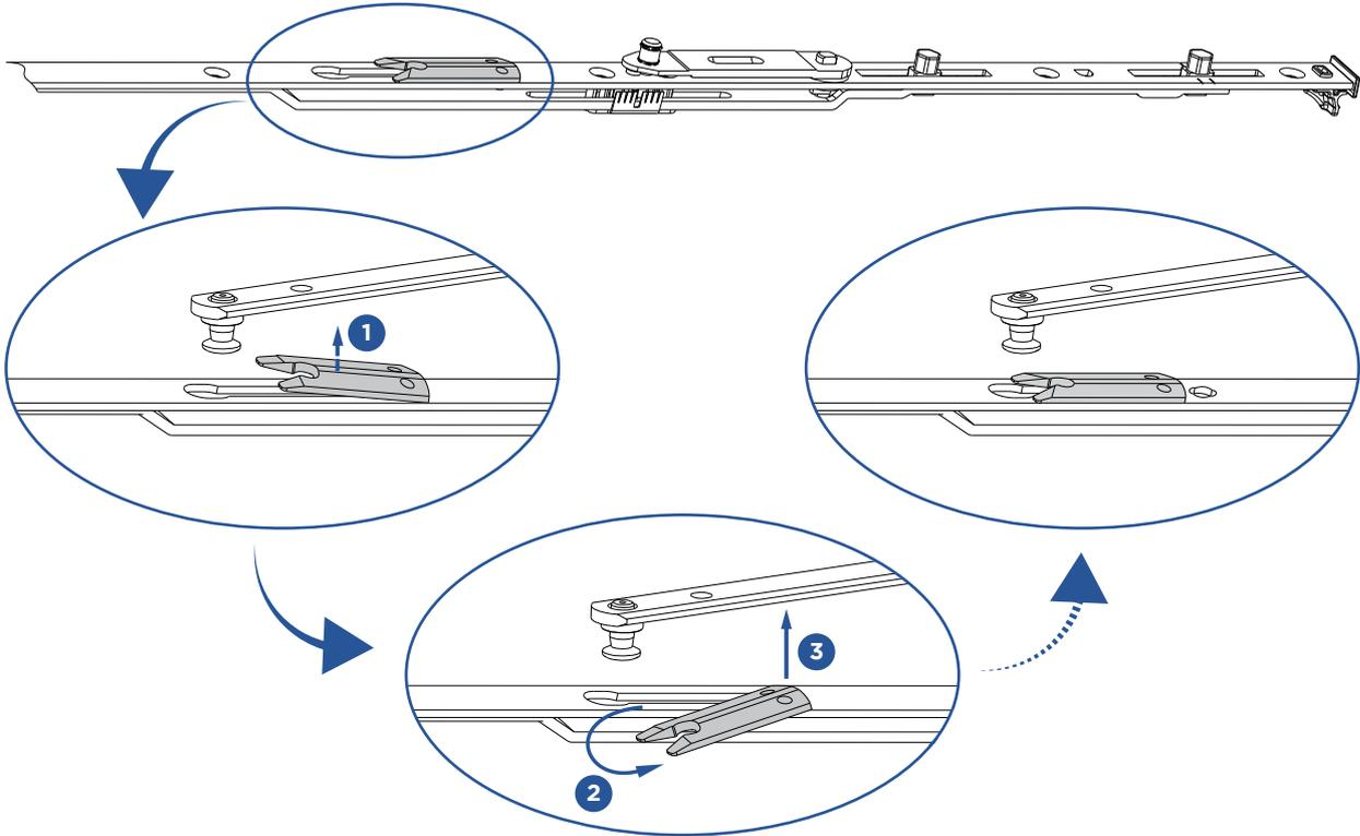
\*PICTURES REPRESENT THE ADJUSTMENT OF THE ANTI-SLAM DEVICE (TILT REDUCEMENT)
