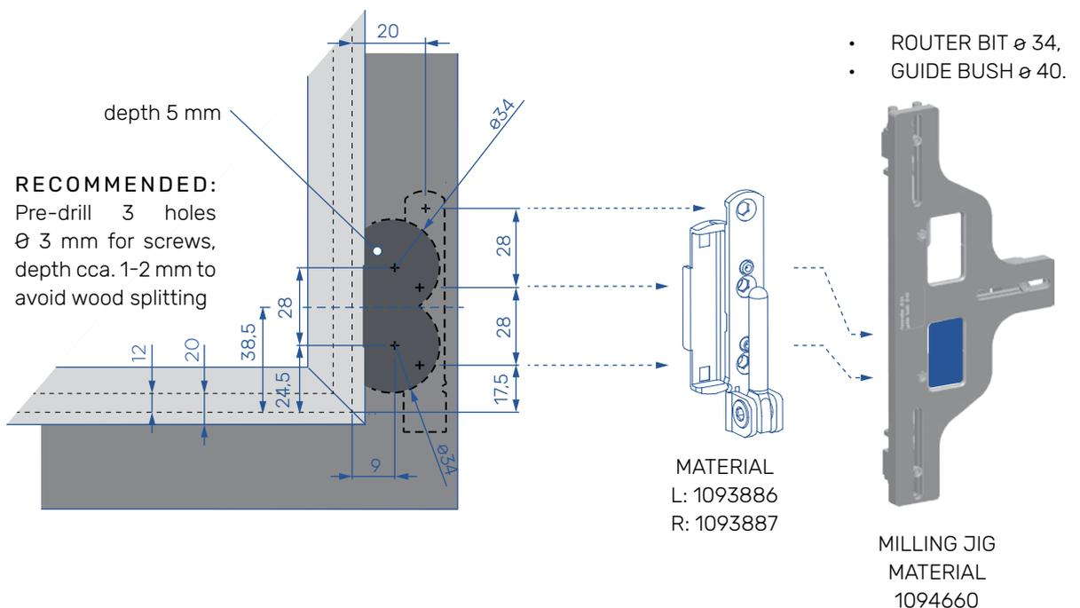
\* READJUST THE MILLING JIG TO 20 mm HARDWARE OVERLAP
