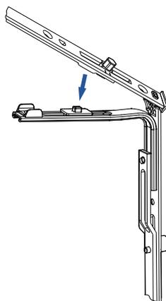
2.) Clamp the hole of a driving rod onto the stay guide connector
