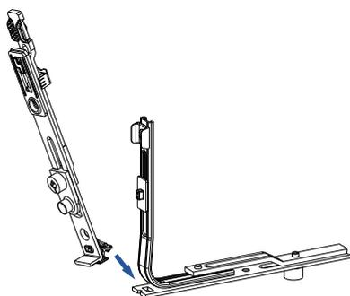
1.) Insert the connecting bracket into the hole of a centre lock
