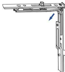
3.) Insert the assembly into a sash groove
