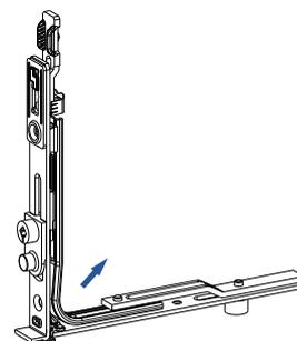
3.) Insert the assembly into a sash groove
