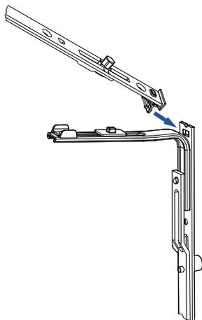
1.) Insert the connecting bracket into the hole of a centre lock
