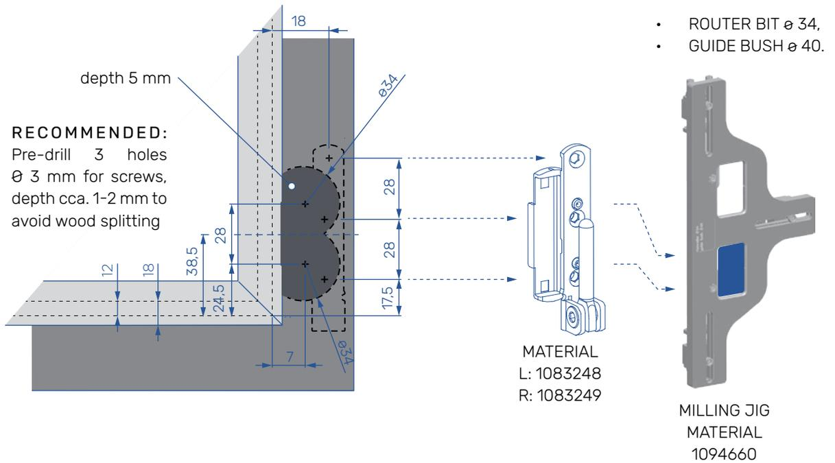
\* READJUST THE MILLING JIG TO 18 mm HARDWARE OVERLAP
