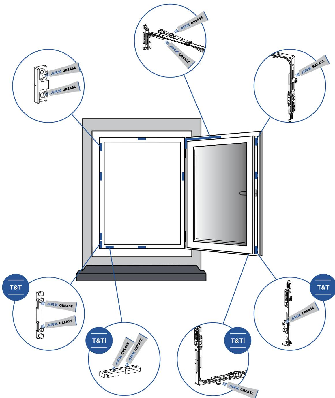
Regular greasing and oiling of operation-relevant components in the sash and frame is recommended at least once a year. In case of frequent use as in schools, hotels the oiling is recommended once in six months.
